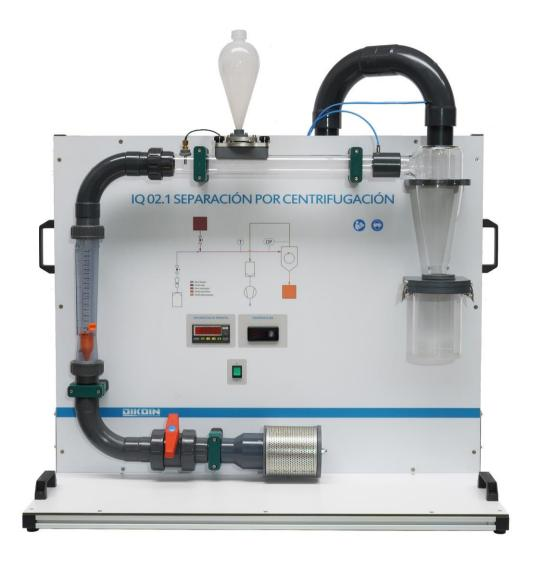
Cyclones are widely used equipment in the industry that allows the separation by centrifugal force of solid particles that are suspended in a gas. They are simple equipments whose operation is based on the separation of the particles by means of the centrifugal force, and that without having movable parts they have a very simple maintenance. As inconvenience we can emphasize that they are not flexible to the changes of concentration, flow or size of the particles.
